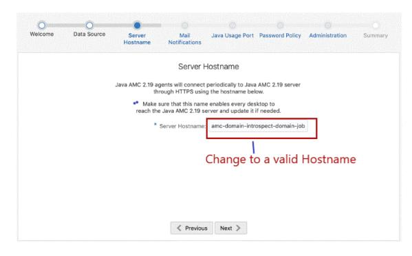
Figure 3-2 Initializing Containerized AMC
